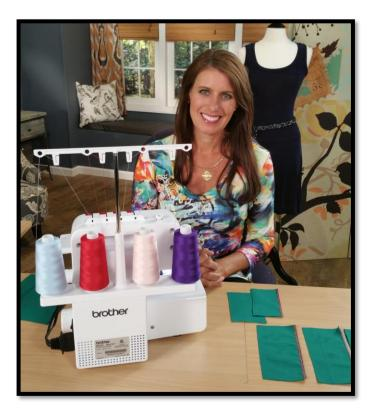
It's a good idea to test serging the fabric you are using for a certain project. An easy way to determine which setting on the serger needs adjusting is to thread the loopers and needles with different colored thread as seen here. Now when you adjust the tension on one setting, you will see the results according to thread color.
